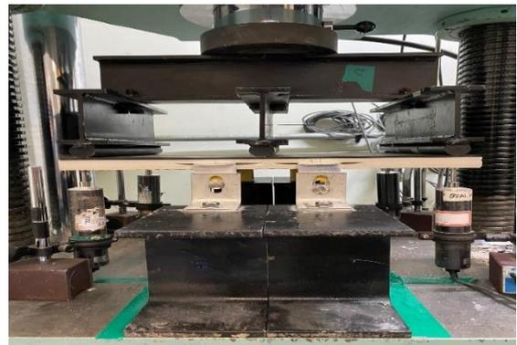
**Fig. 1 Direct Shear Test Model Dimension and Test Setup**
